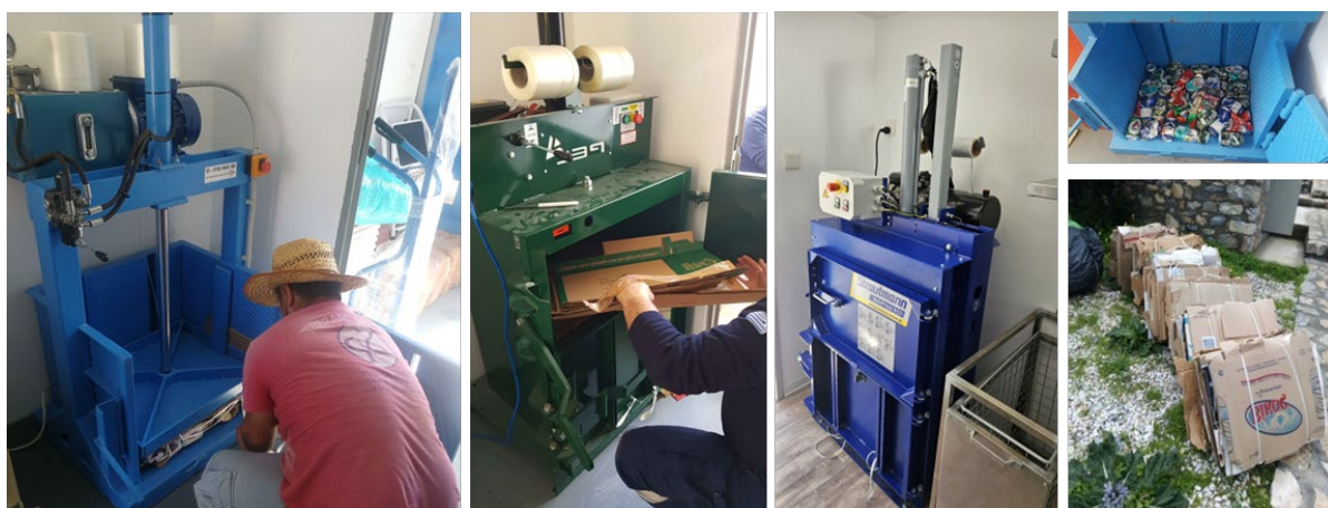
Figure 5 Compressing and bailing of the material
